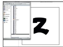
Repeat this procedure until you have all the letters for your alphabet. Save each letter as an *Illustrator 3* EPS file, and name each letter accordingly. Remember to remove the guides before saving each letter: you can use Edit>Undo to reinstate the guides quickly, rather than reopening the base eps file each time.
